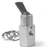
**0811** Normally closed toggle valve for air control. The detent switches release the air going to your cylinders so that they can return to their closed position. They fit nicely into a control panel and include the nuts for mounting. Thread size of the ports is 10/32 male. You will need to also order the proper fitting to go to the hose you are using .
